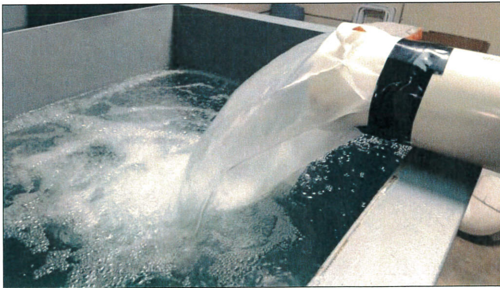
Figure 4. Net at effluent pipe discharge.
